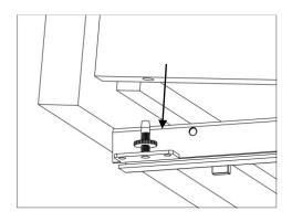
Place drawer box on top of drawer glide; ensure the hole on drawer is mounted onto the pin of the glide. The pins at the rear of the tracks should align with holes in the back of the drawer box. The height of the drawer can be adjusted by turning the balancer on the pin.
